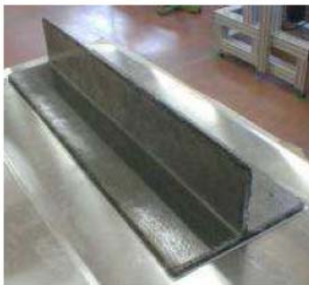
'T' beam in composites
