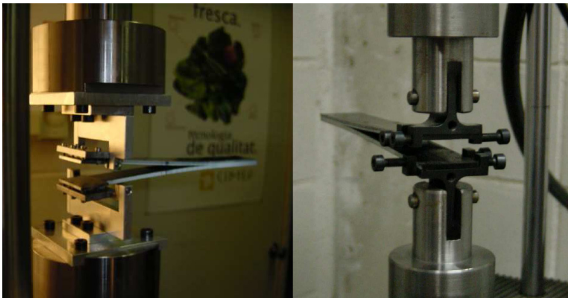
Figure 1- The new tools during a DCB test.
