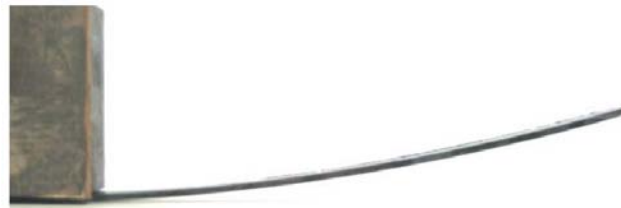
Figure 3- Cross-ply composite at room temperature after curing at 180°.
