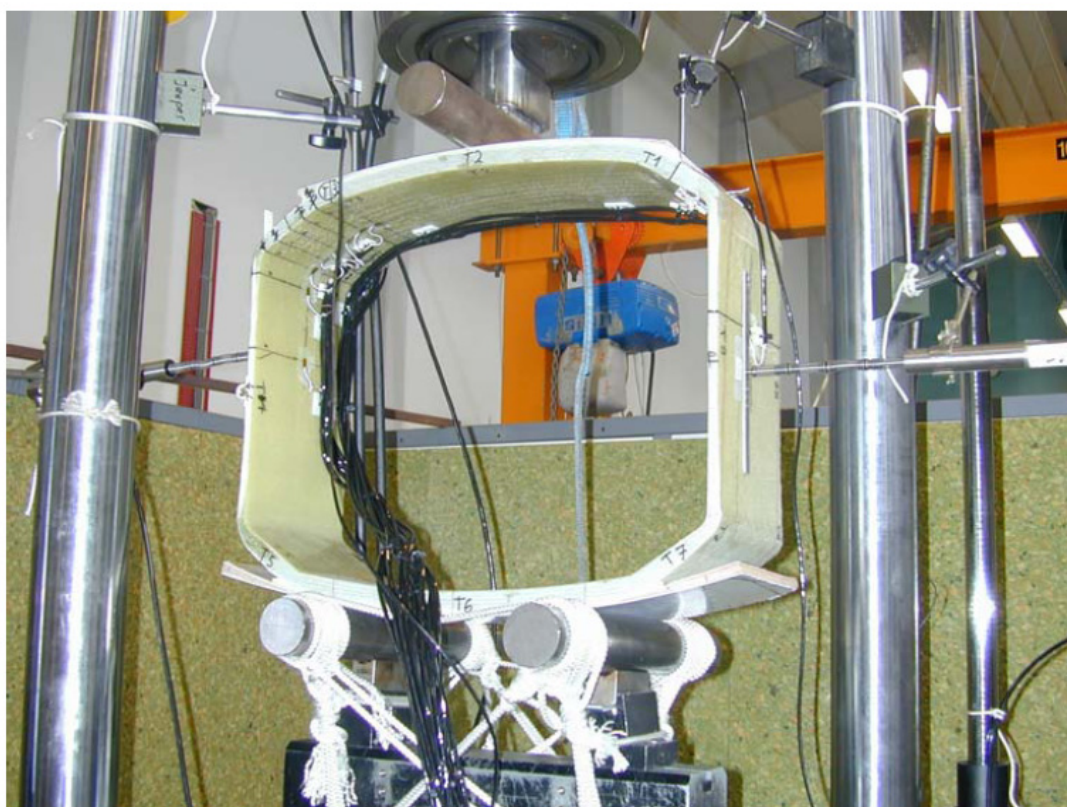
Figure 1- Test setup. The top is fixed and the bottom with the two supports is moving upward during loading.
