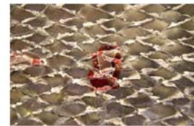
Figure 1- Strain gage failure
