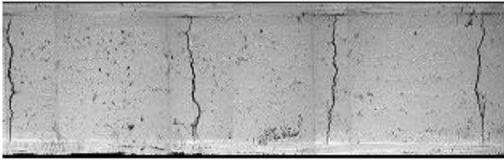
a) intralaminar cracks
