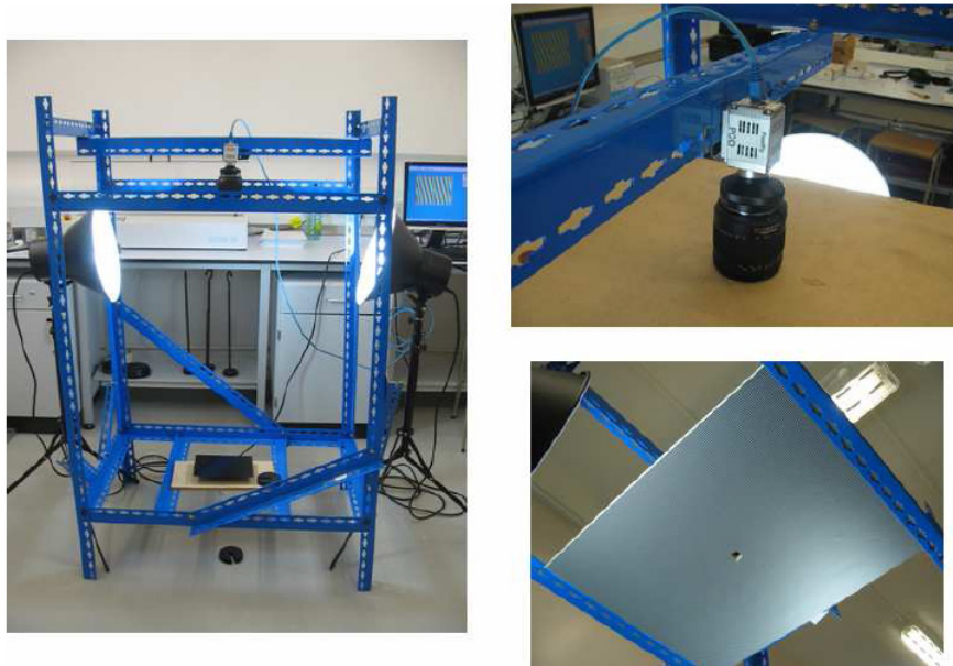
Figure 3- General view of the deflectometry set-up, camera and grating.
