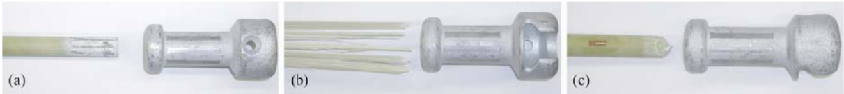
Figure 2- Failure mode depending on the crimping pressure: (a) sliding, (b) delamination, or (c) fracture.
