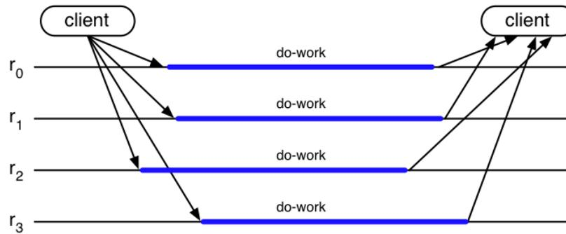
**Figure 11.9.** Active replication (adapted from [Guerraoui and Schiper 1997])
