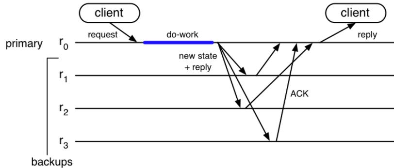
**Figure 11.8.** Primary-backup replication (adapted from [Guerraoui and Schiper 1997])
