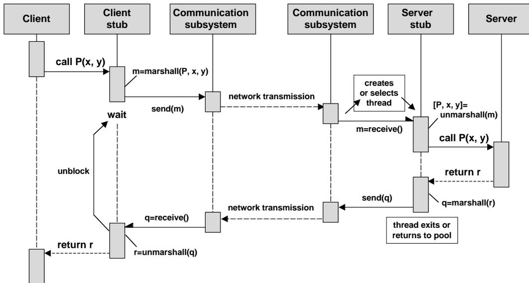
Figure 1.9. Remote procedure call: overall flow of control
