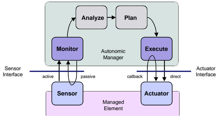
Figure 10.8. Interfaces for sensors and actuators
