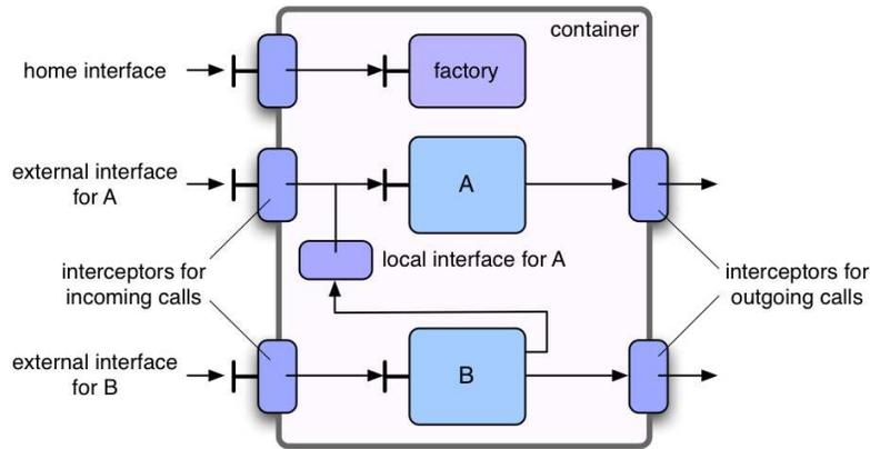
Figure 7.13. Container-mediated communication
