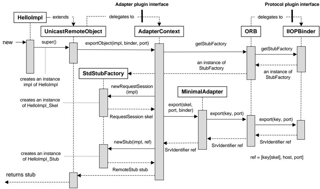
**Figure 5.15.** Remote Method Invocation: creating the stub and skeleton
