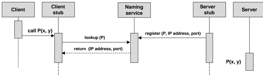
**Figure 1.10.** Remote procedure call: locating the server
