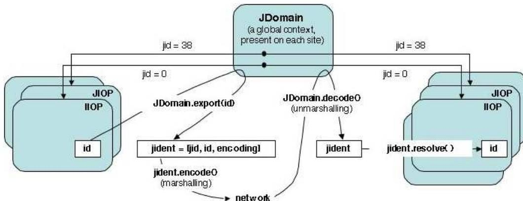
Figure 3.18. Transmitting an identifier over a network
