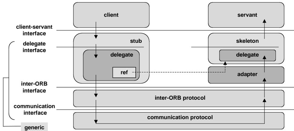
**Figure 5.6.** The invocation path and its main interfaces
