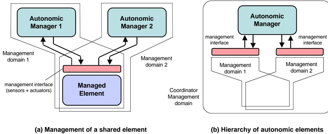
Figure 10.7. Multiple domains for autonomous management
