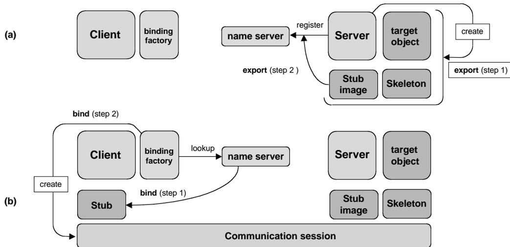
**Figure 3.15.** Using the `export-bind` pattern for client-server binding
