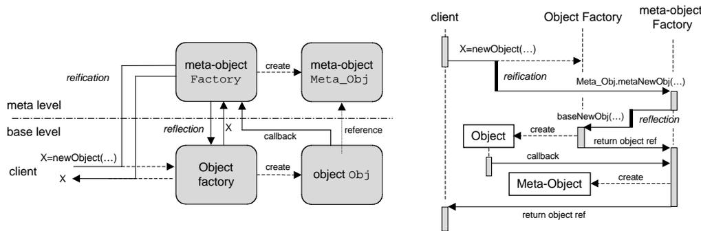
Figure 2.15. Object creation in a reflective system
