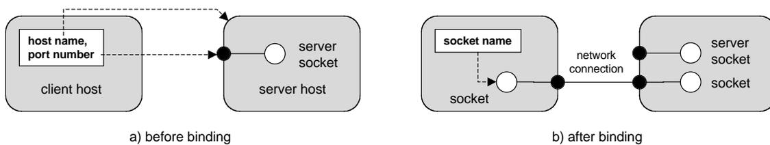
Figure 3.11. Client to server binding using sockets
