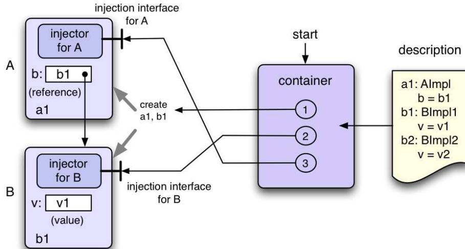
Figure 7.11. Inversion of control: interface injection
