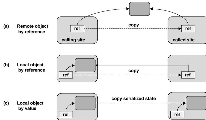
Figure 5.8. Passing an object as a parameter
