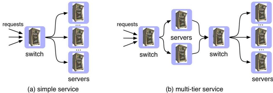
Figure 12.3. Load balancing
