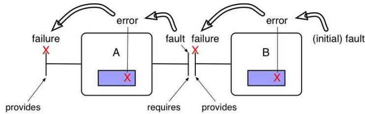
Figure 11.2. Error propagation
