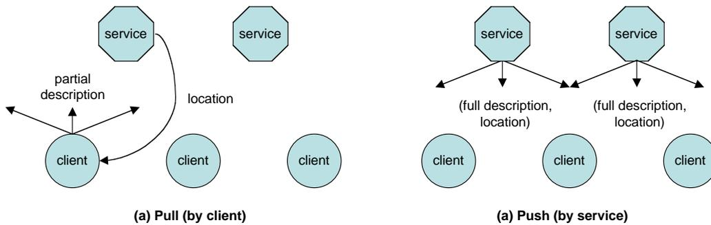
Figure 3.9. Interaction patterns for service discovery (without servers)
