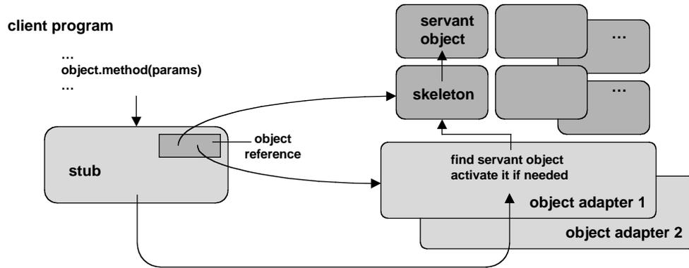
Figure 5.7. Invoking a remote object through an adapter
