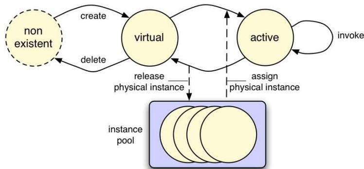
**Figure 7.12.** Instance pooling
