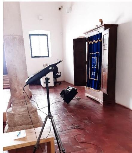
**Figure 7.** Sound source and sound level meter to perform RT measurements.
