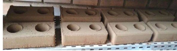
Figure 1: Bricks in curing process
