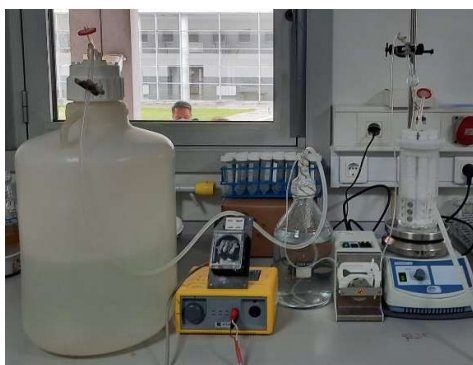
Figure 14: Experimental installation for biofilm growth using the CDC reactor.
