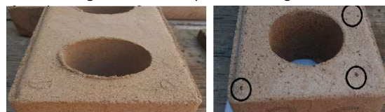
Figure 2: Visible granules of sludge
