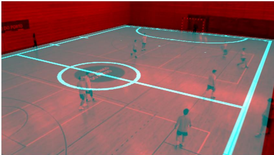
Figure 4.8: Model of the field projected on the first frame using the initial homography
