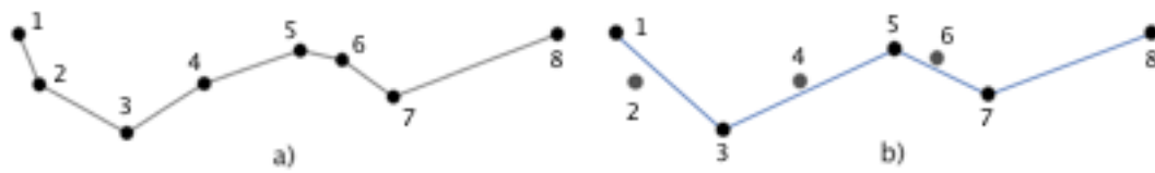
Figure 3.7: Smoothing a piecewise linear curve with the Douglas–Peucker algorithm.
