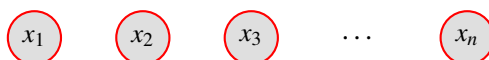
Figure 4.6: A factor graph modelling a uniform distribution over the sensed set of features x .
