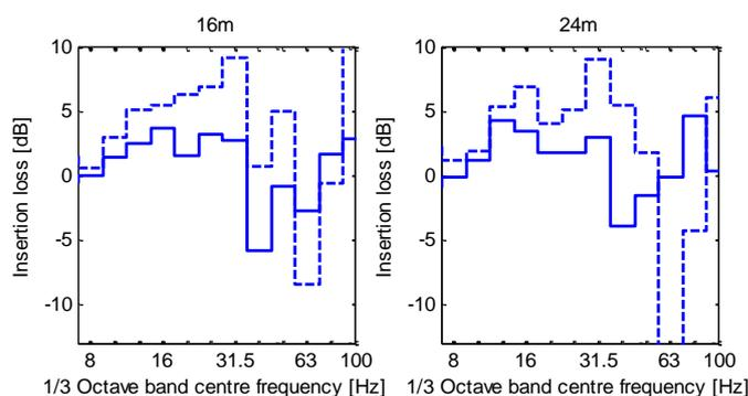
Figure 16. Insertion losses at Lincent, 6 m wide wave impeding blocks. Solid line: thickness of the block is 0.5 m, depth to the top of the block in the soil 0.9 m; Dashed line: thickness of the block is 1 m, depth to the top of the block in the soil 0.4 m. Response to a line source. Corrected for vehicle/track interaction
