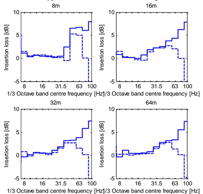
Figure 5. Insertion loss for subgrade stiffening, at Horstwalde without (solid line) and with (dashed line) track.
