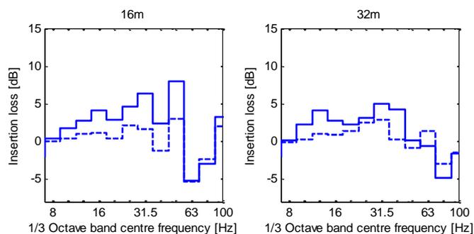
Figure 8. Insertion loss at Lincent, concrete (solid line) and jet grouting (dashed line). Response to a line source. Corrected for vehicle/track interaction.
