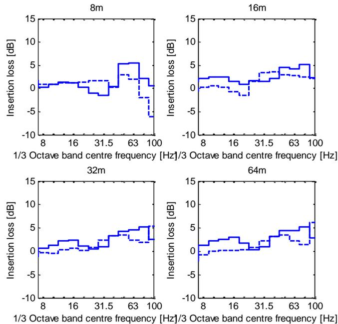
Figure 11. Insertion loss for wave impeding block at Horstwalde without (solid line) and with (dashed line) considering track. Response to point load (uncorrected).
