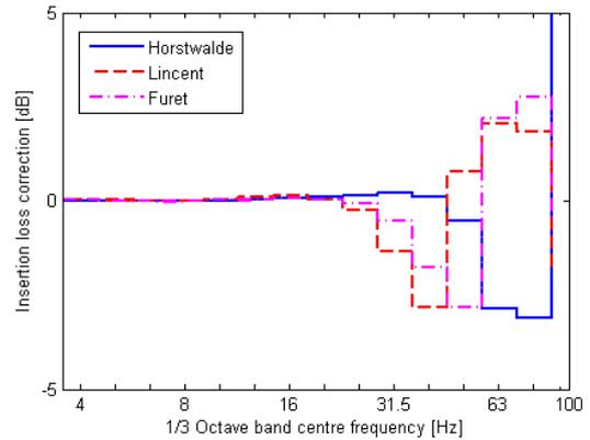
Figure 12. Insertion loss correction due to vehicle/track interaction for wave impeding blocks at the reference sites.
