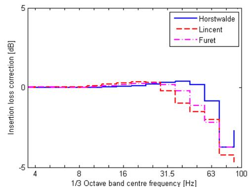
Figure 6. Insertion loss correction due to vehicle/track interaction for subgrade stiffening at the reference sites.
