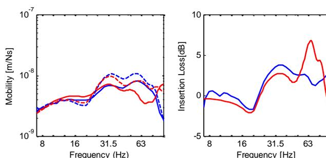
Figure 3 Transfer mobility (3a) and insertion loss (3b) for a point load at a distance of 16 m for a wave impeding block (6 m wide, 0.5 m thick, 0.9 m deep) at the Horstwalde site. Solid line: with subgrade stiffening, dashed line: without subgrade stiffening. ISVR (red), KU Leuven (blue).
