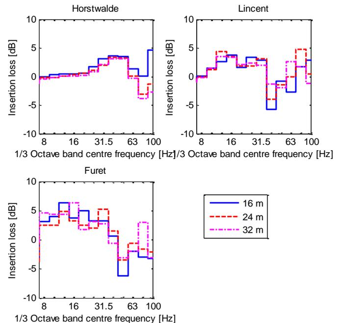
Figure 13. Effect of soil conditions on the insertion loss resulting from a wave impeding block. Responses at 16 m (blue solid line), 24 m (red dashed line) and 32 m (purple dash-dot line).
