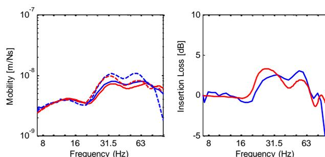
Figure 2 Transfer mobility (2a) and insertion loss (2b) for a point load at a distance of 16 m for subgrade stiffening (6 m wide, 0.5 m high) at the Horstwalde site. Solid line: with subgrade stiffening, dashed line: without subgrade stiffening. ISVR (red), KU Leuven (blue).
