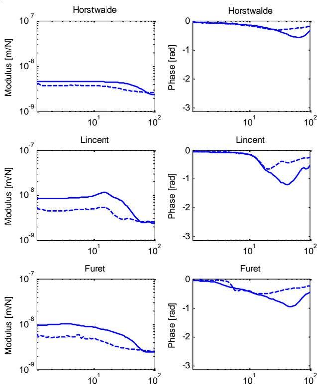
Figure 4. Track receptance with and without subgrade stiffening at the three reference sites. Solid line: without subgrade stiffening, dashed line: with subgrade stiffening.
