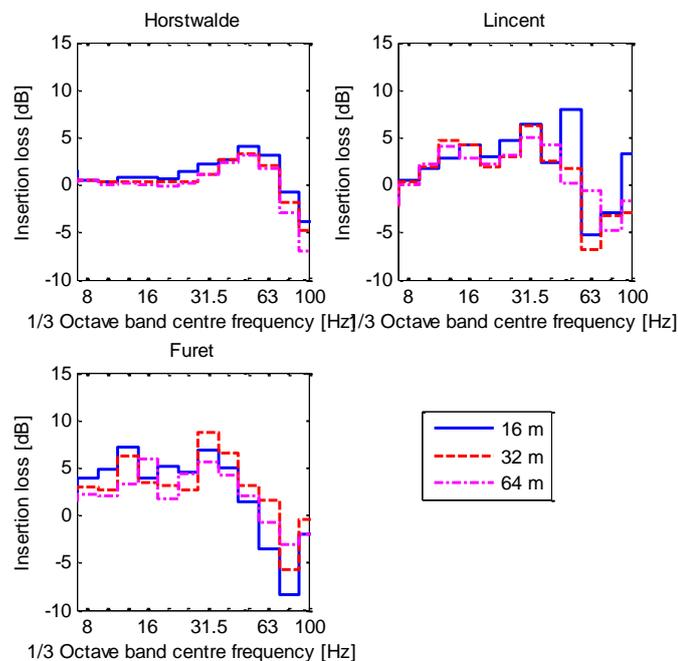
Figure 7. Effect of soil conditions on the insertion loss resulting from subgrade stiffening. Responses at 16 m (blue solid line), 24 m (red dashed line) and 32 m (purple dash-dot line) to a line source. Corrected for vehicle/track interaction.
