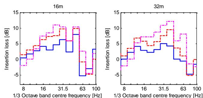
Figure 9. Effect of block thickness on the insertion loss of subgrade stiffening for Lincent: 0.5 m thick (blue solid line), 1 m thick (red dashed line) and 2 m (purple dash-dot line).
