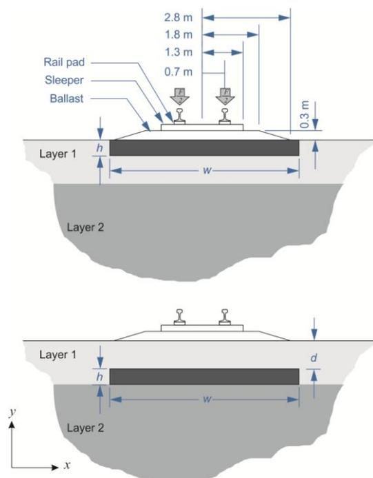
Figure 1. Example sketch of track section at layered soil site of Lincent with soil stiffening (top) and wave impeding block (bottom)
