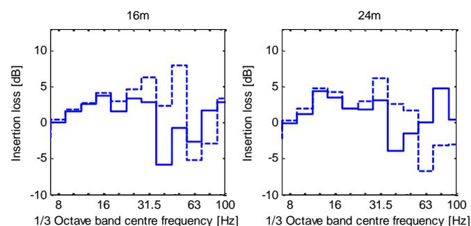
Figure 17. Insertion losses at Lincent, concrete block with width of 6 m in width and thickness of 0.5 m. Solid line: wave impeding block, depth to the top of the block in the soil 0.9 m; Dashed line: subgrade stiffening, depth to the top of the block in the soil 0 m. Response to a line source. Corrected for vehicle/track interaction.
