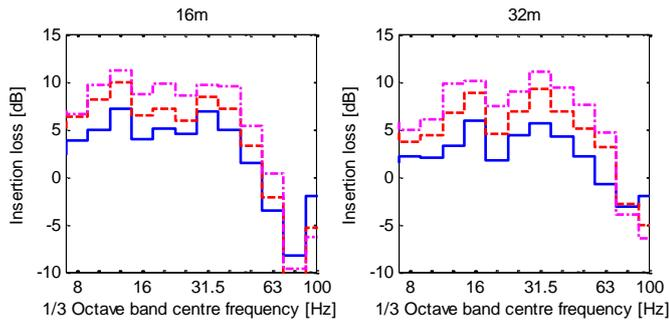
Figure 10. Effect of block thickness on the insertion loss of subgrade stiffening for Furet: 0.5 m thick (blue solid line), 1 m thick (red dashed line) and 2 m (purple dash-dot line).
