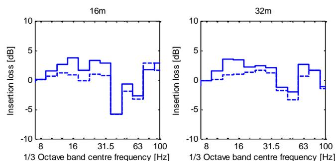
Figure 14. Insertion losses at Lincent, wave impeding blocks, using concrete (solid line) and jet grouting material (dashed line). Response to a line source. Corrected for vehicle/track interaction
