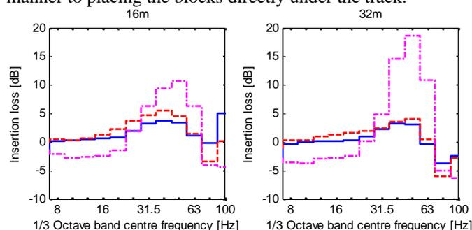
Figure 15 Insertion losses at Horstwalde, wave impeding blocks with widths of 6 m (blue solid line), 12 m (red dashed line) and infinite (purple dot-dash line). Response to a line source. Corrected for vehicle/track interaction.
