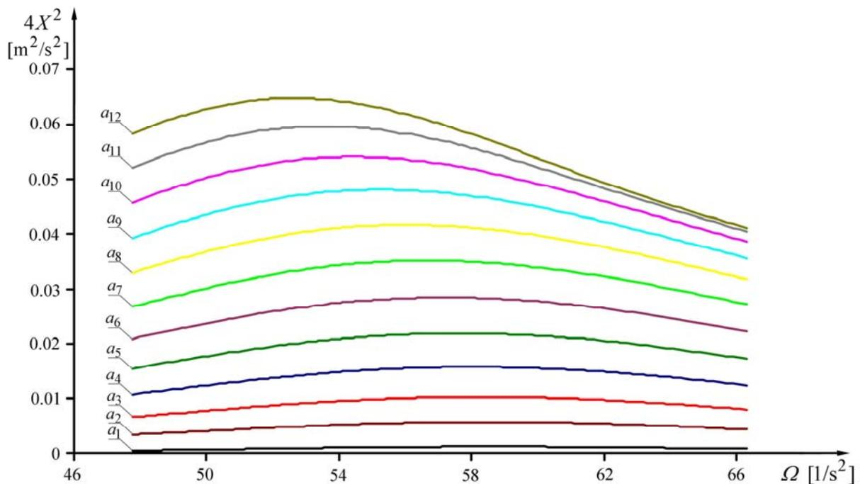
Figure 9. Special frequency characteristics of the relative displacements for the mass  $m$ .
