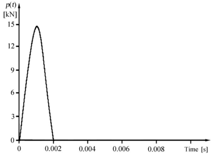
Figure 5. Example of the applied shock loads.
