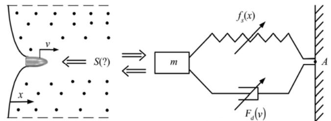
Figure 1. Conceptual model of the piercing process.
