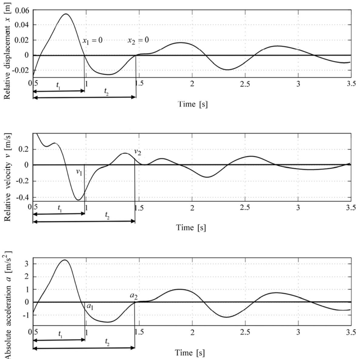
Figure 6. Example of the free vibrations of the mass  $m$  of the tested system.
