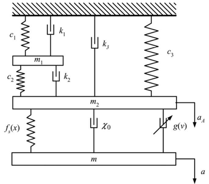
Figure 3. Scheme of the tested system.
