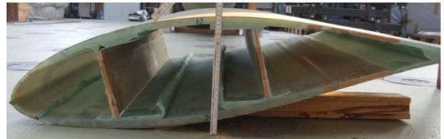
Figure 6: Cross-section of a rotor blade with manufacturing faults
