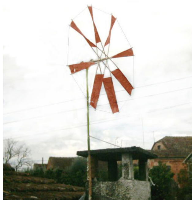
Fig. 16 A model of a 1 m diameter convergent turbine built of wood sticks and blades made of TESA ® adhesive tape.
