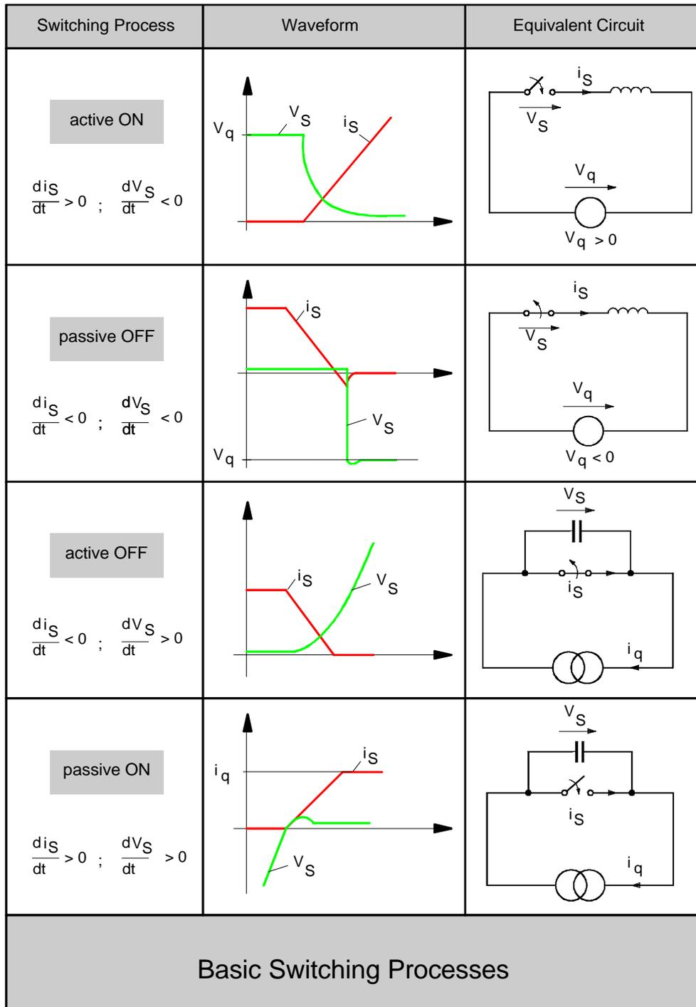
Figure 0.3 Basic switching processes
