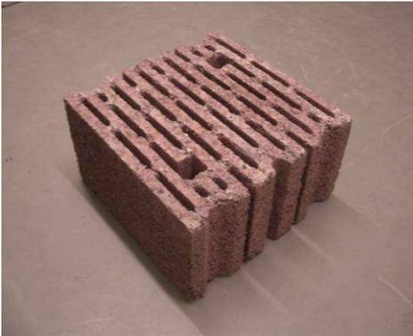
**Figure 9.** Lightweight concrete block of expanded clay developed in the OTMAPS project
