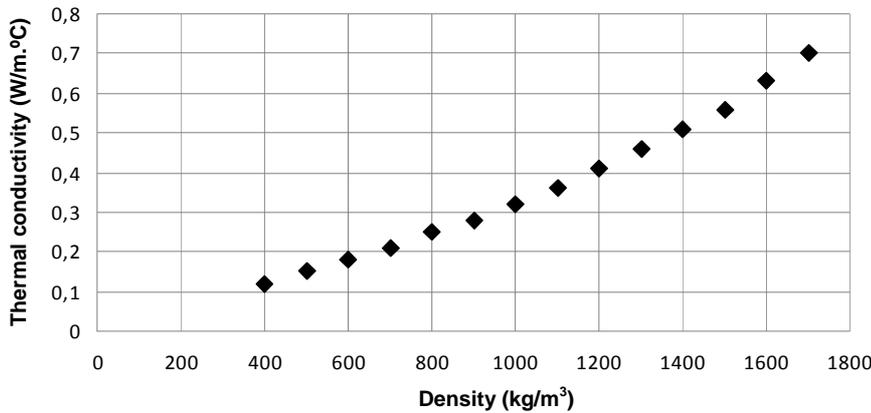
**Figure 2.** Thermal conductivity versus apparent density of a lightweight concrete with expanded clay aggregates [5]
