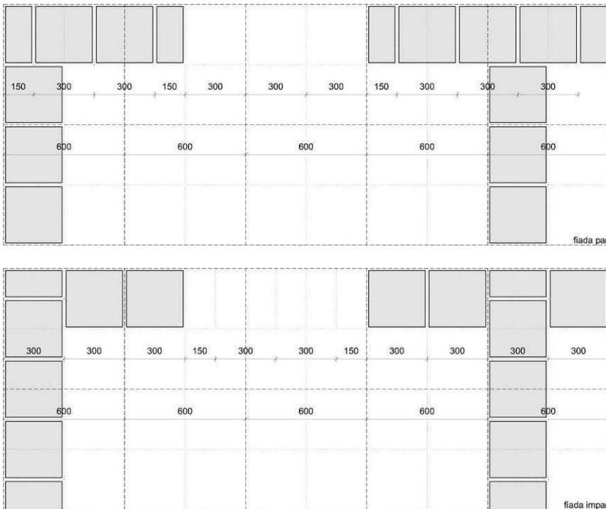
Figure 7. Example of modular system coordination in masonry
