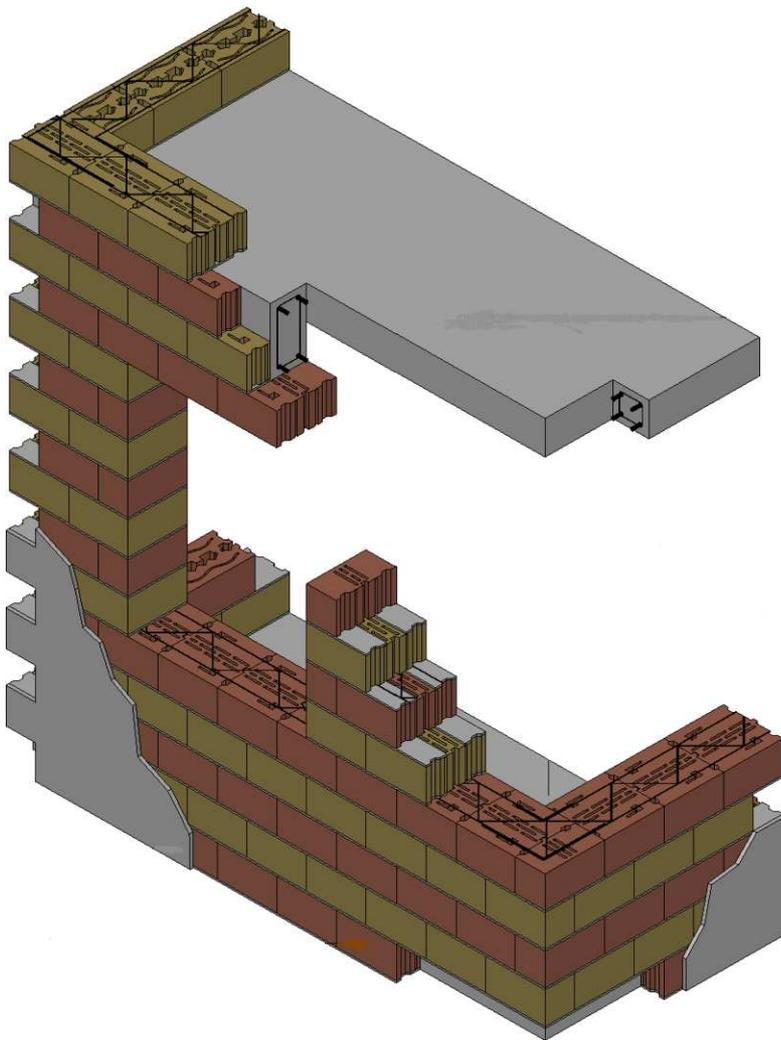
**Figure 8.** Axonometric projection of a reinforced masonry system
