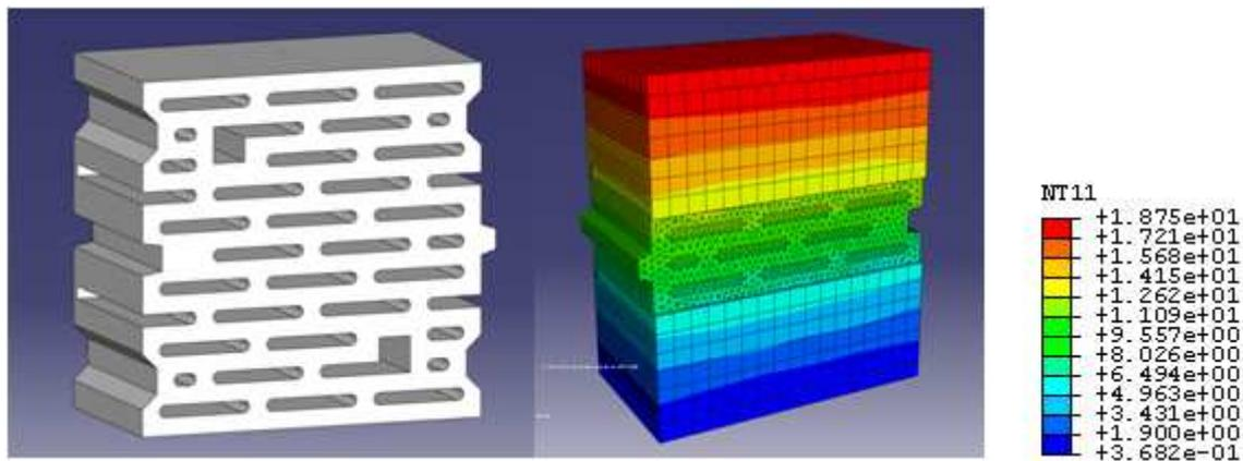
**Figure 4.** Distribution of temperatures in rendered block for optimal design solution based on external and internal temperatures of 0°C and 20°C respectively
