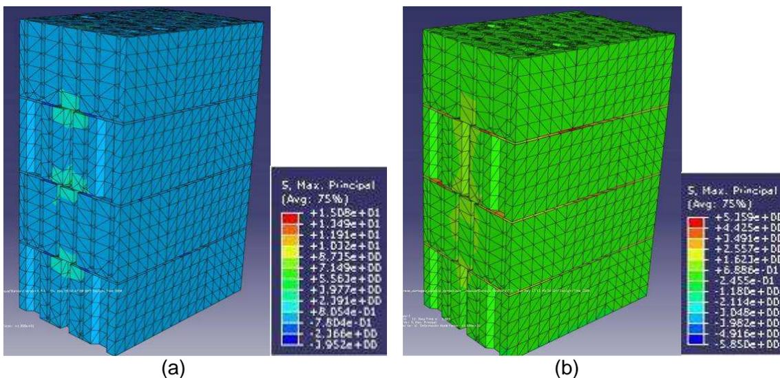
**Figure 5.** Numerical simulation of stresses (MPa) in a wall with four rows of blocks loaded according tests results: (a) elastic analysis; (b) elasto-plastic analysis
