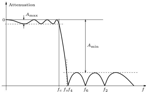
Figure 5: Frequency response of a seventh-order Cauer-Chebyshev filter
