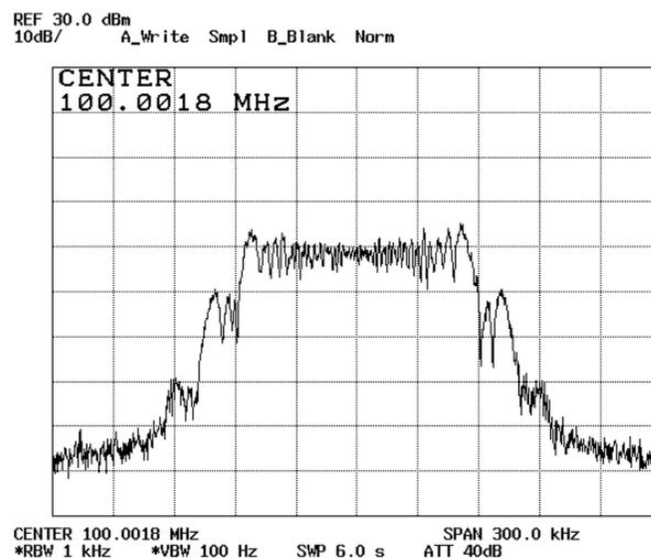
(b) modulated with a 1kHz sine wave at 0 dBFS
