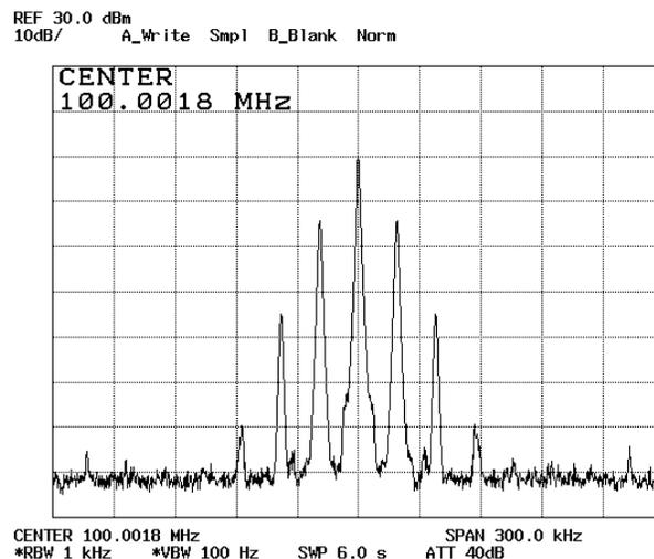
(a) unmodulated carrier (19 kHz pilot tone only)
