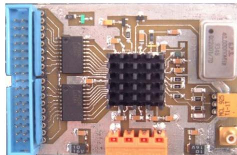
Figure 4: Direct digital synthesizer board
