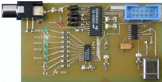
Figure 3: S/PDIF interface board
