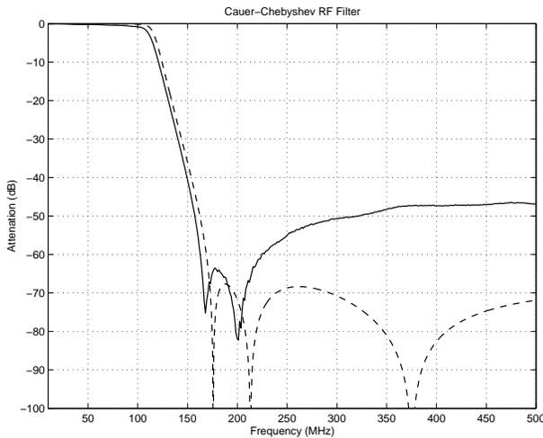
Figure 7: Actual and simulated filter frequency responses
