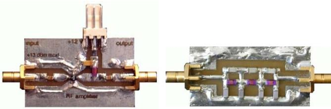
Figure 8: PCB images of the designed filter and amplifier (left image)
