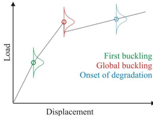
Figure 1: Sketch of the load-displacement curve of a stringer dominated stiffened panel under axial compression
