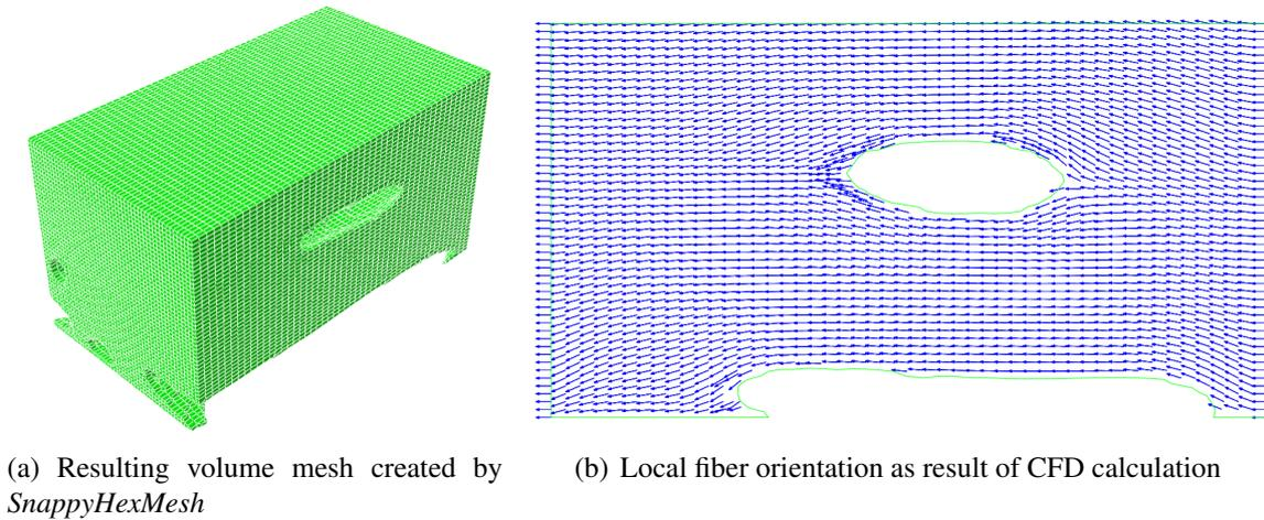
Figure 1. Determination of local fiber undulation
