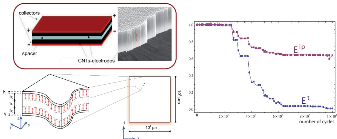
Figure 1. Supercapacitor scheme (left) and elastic moduli reduction vs. number of cycles.
