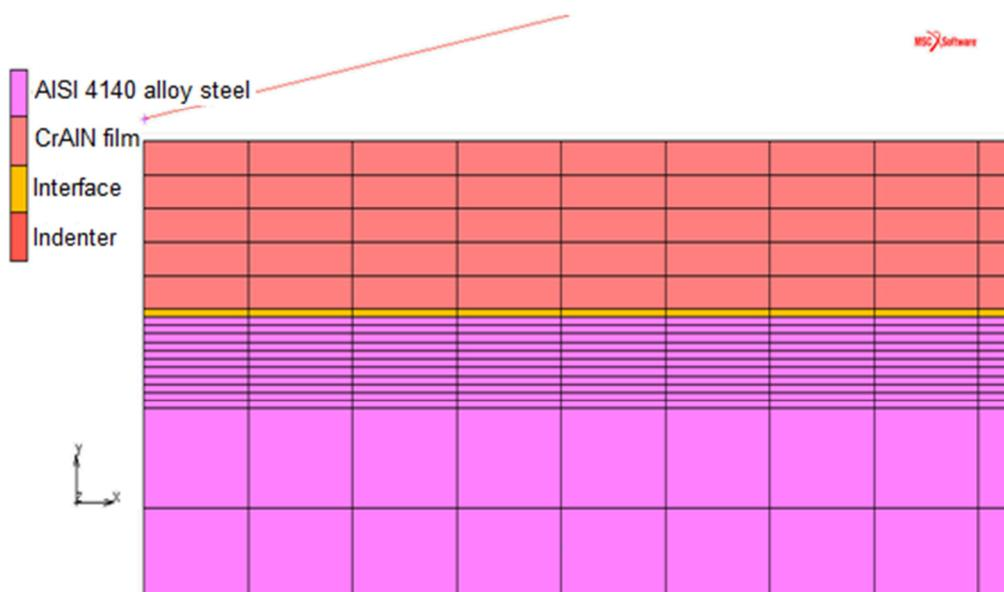
Fig. 2 - Numerical mesh at the contact region of spherical indentation testing in a system with film, interface and substrate
