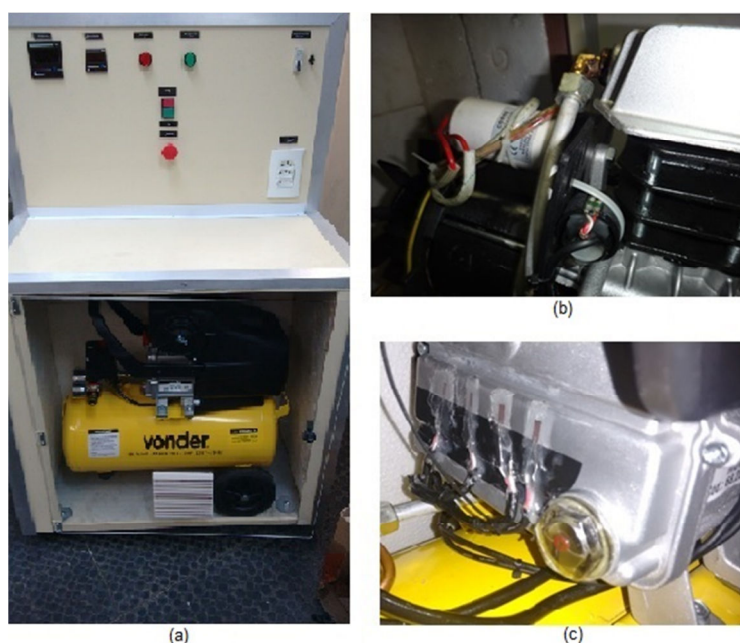
Fig. 1 - Test bench with transducers. (a) Shows the test bench; (b) coupled microphone; (c) the strain gauges on oil plate.
