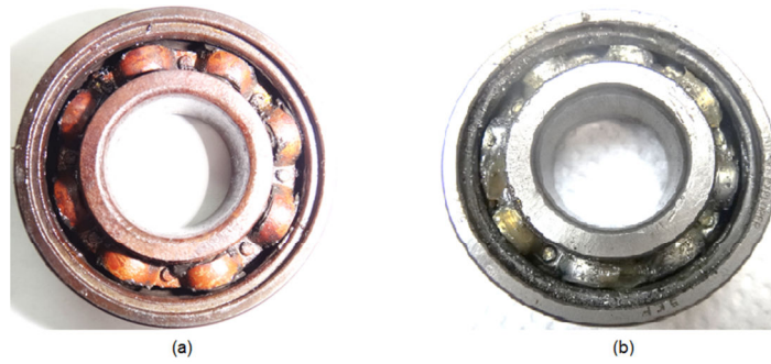
Fig. 2 - Tribological failures in 6202 bearing. (a) Corrosion and (b) debris.
