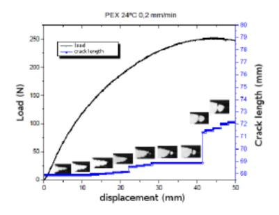
Fig. 1 - Constant rate test on DCB sample
