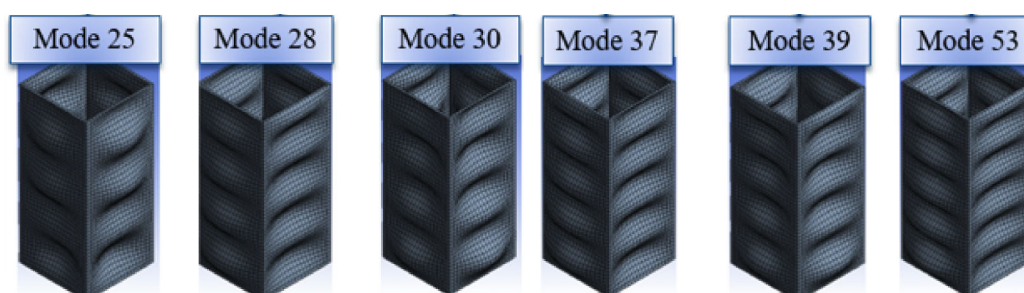
Fig. 2 - Drawings of the deformation patterns associated to the selected buckling mode shapes calculated for the structure of this case study. Some of the modes (28, 37, 53) include concave and convex profiles in the same cross section (mixed mode), while other modes (25, 30, 39) include either concave or convex profiles (independent mode).
