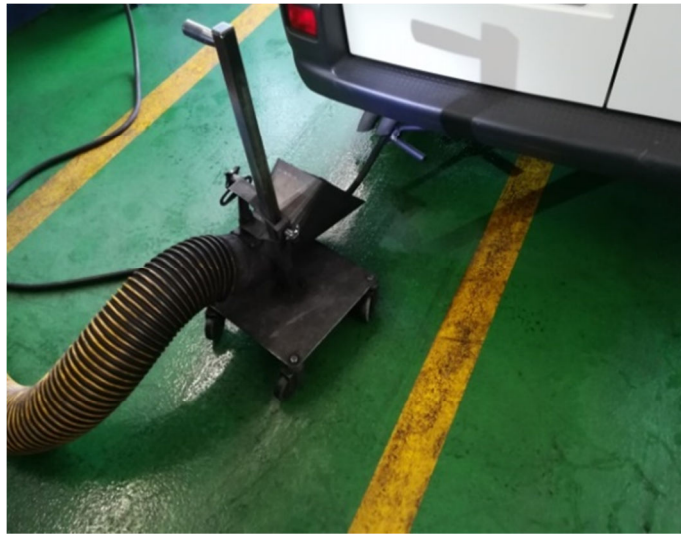
Fig. 4 - Emission control in a PTI station. Source: SYC-APPLUS
