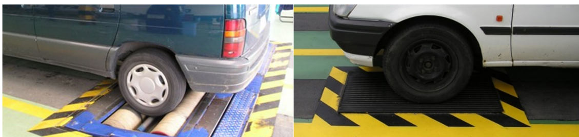
Fig. 1 - Roller Brake Testers (left) and a Side Slip Testers (right). Source: SYC-APPLUS
