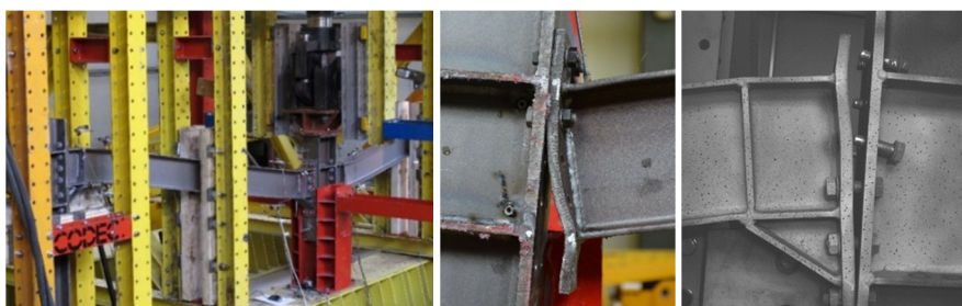
Fig. 1 - Experimental test set-up and column loss test results
