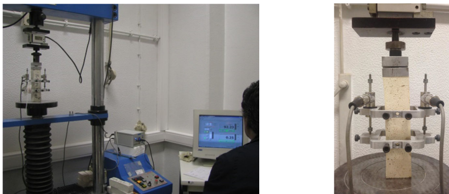
Fig. 6 - instrumented test specimen for a static E test
