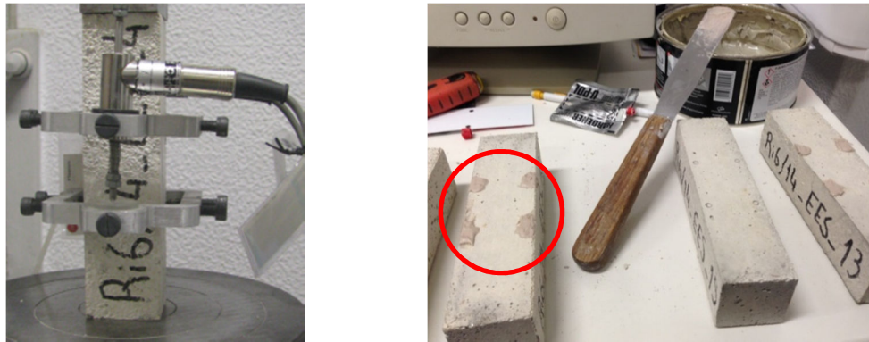
Fig. 5 - (left) displacement transducer used and (right) reinforced areas of a test specimen
