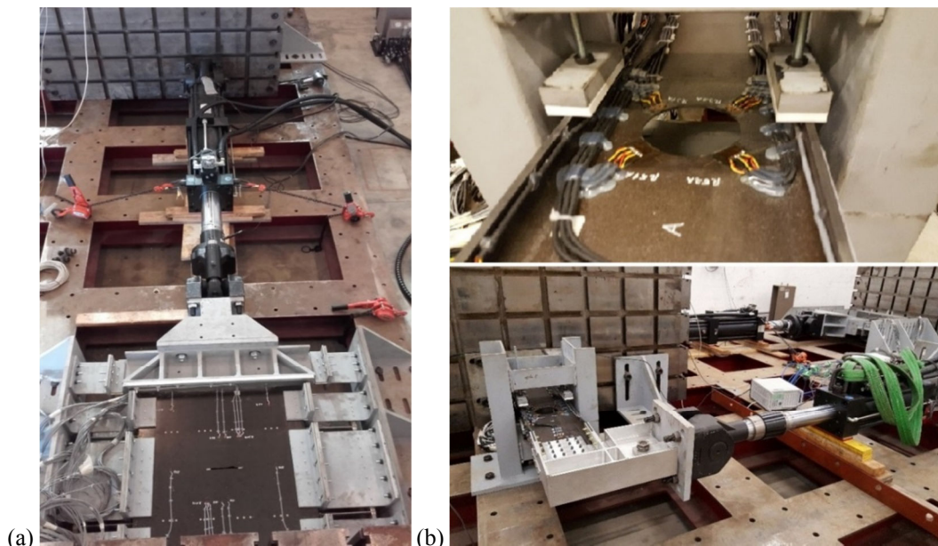
Fig. 11 - Final layout of the multi-stringer component compression test (a) and of static spar test with the anti-buckling structure (b).
