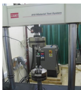
Fig. 2 - Characterization of the MR damper (RD-1005-3) on traction machine 'MTS 810'
