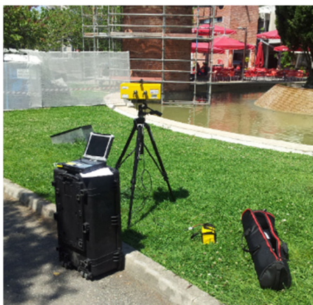
Fig. 1 - View of the radar interferometer from (Silva, 2015).
