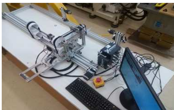
Fig. 2 - Filament Winding Equipment used by the University of Aveiro
