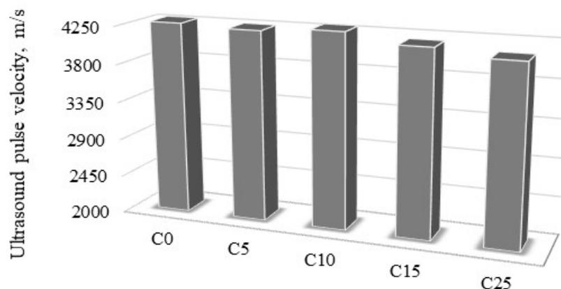
Fig. 7 - The results of concrete ultrasound pulse velocity after 28 days curing
