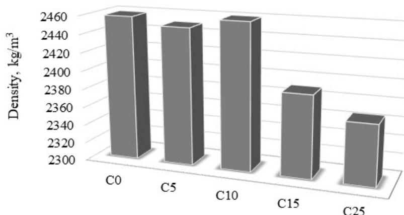
Fig. 6 - Density of concrete with 0, 5, 10, 15 and 25% (w/w) of cement replacement with FCCCW catalyst after 28 days curing
