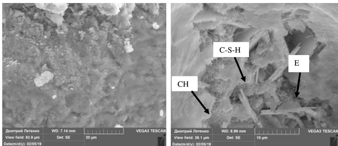
Fig. 9 - Images of microstructure C10 after 28 days (Note: CH-portlandite; E-ettringite; C-S-H-calcium silicate hydrate)
