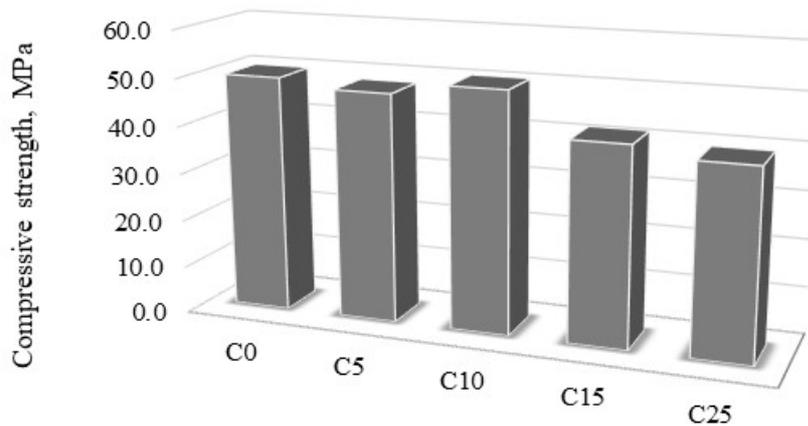
Fig. 5 - Compressive strength of concrete with 0, 5, 10, 15 and 25% (w/w) of cement replacement with FCCCW catalyst at 28 days of age
