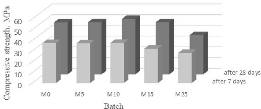
Fig. 2 - Compressive strength of mortars with 0, 5, 10, 15 and 25% (w/w) of cement replacement with FCCCw catalyst at 7 and 28 days of age
