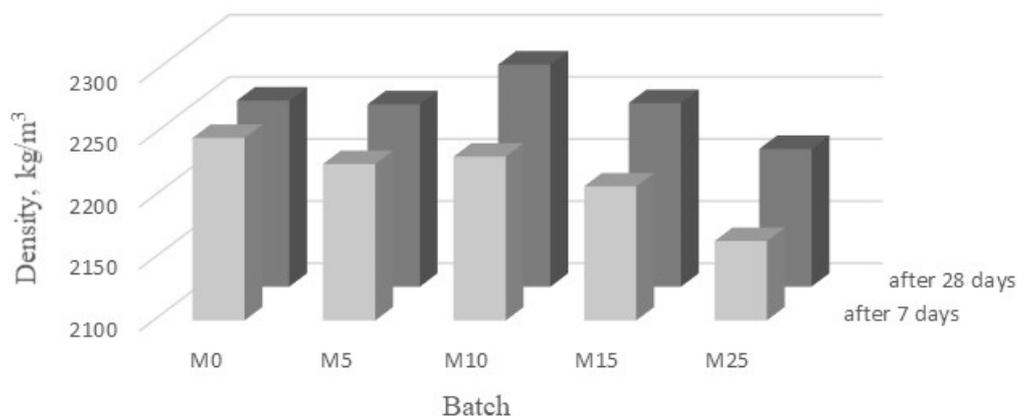
Fig. 3 - Density of cement mortars with 0, 5, 10, 15 and 25% (w/w) of cement replacement with FCCCw catalyst after 7 and 28 days curing
