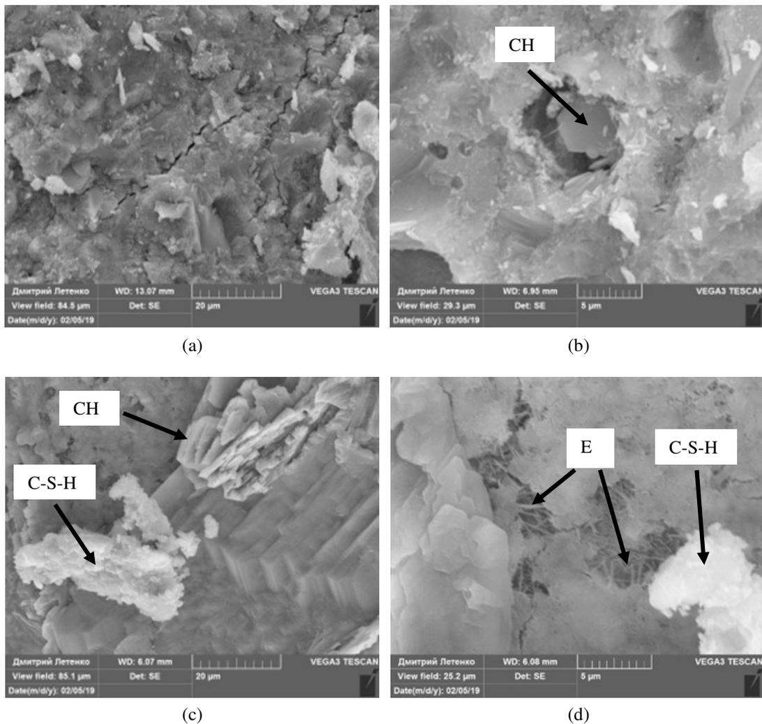
Fig. 8 - Images of the microstructure of concretes without and with 5% of FCCCW incorporation obtained on a fractured surfaces: (a), (b) C0; (c), (d) C5 (Note: CH-portlandite; E-ettringite; C-S-H - calcium silicate hydrate)
