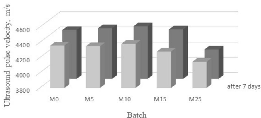
Fig. 4 - The results of cement mortar ultrasound pulse velocity after 7 and 28 days curing
