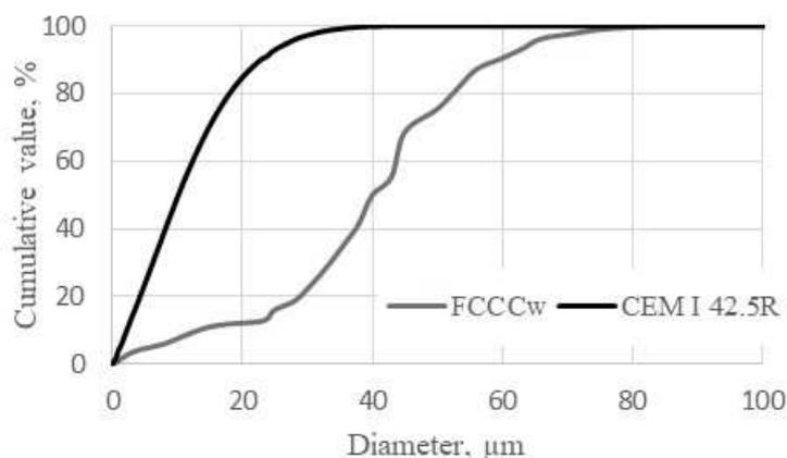
Fig. 1 - Particle size distributions of cement and FCCCw
