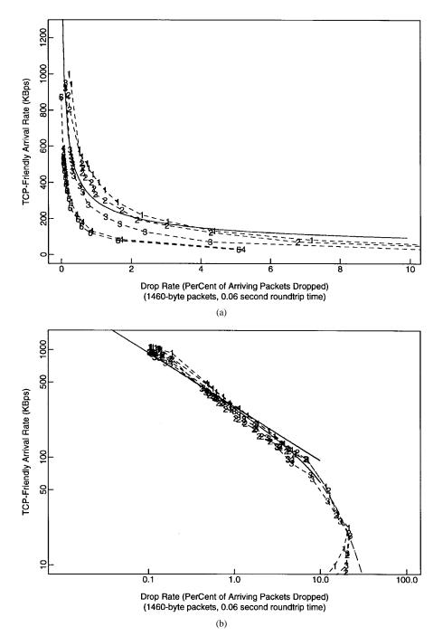
Fig. 10. TCP-friendly bandwidth for a 60-ms round-trip time and 1460-byte packets.
