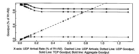
Fig. 5. Simulations with three TCP flows and one UDP flow, with WRR scheduling. There is no congestion collapse.
