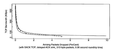
Fig. 11. TCP bandwidth versus steady-state drop rate, for SACK TCP with a delayed-ACK receiver, a 60-ms round-trip time and 512-byte packets.
