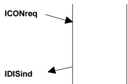
Figure 1.3c Unsuccessful connection establishment (erroneous transmission of the connection request)
