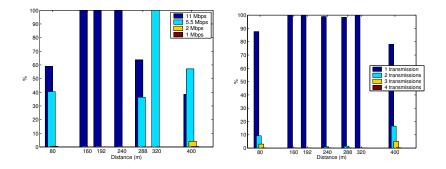
The left histogram shows the rates at which each frame was sent, the right one is the number of retransmissions at each distance. VoIP quality in this scenario is generally good.
