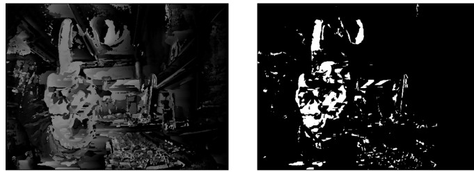
Figure 3.7: Disparity map using SAD over a 5 \times 5 window and its thresholded version.
