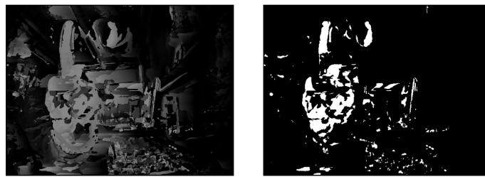
Figure 3.8: Disparity map using SAD over a 7 \times 7 window and its thresholded version.
