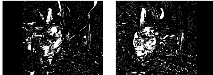
Figure 3.13: Bitmaps produced by merging SAD and CENSUS results of both sweeps. LR sweep outcome on the left, RL on the right.
