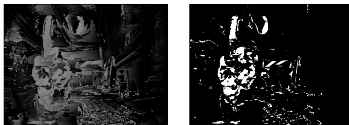
Figure 3.6: Disparity map using SAD over a 5 \times 3 window and its thresholded version.
