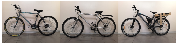
(A) diamond, steel frame. (B) diamond, aluminum (C) narrow diamond, aluminum frame.
