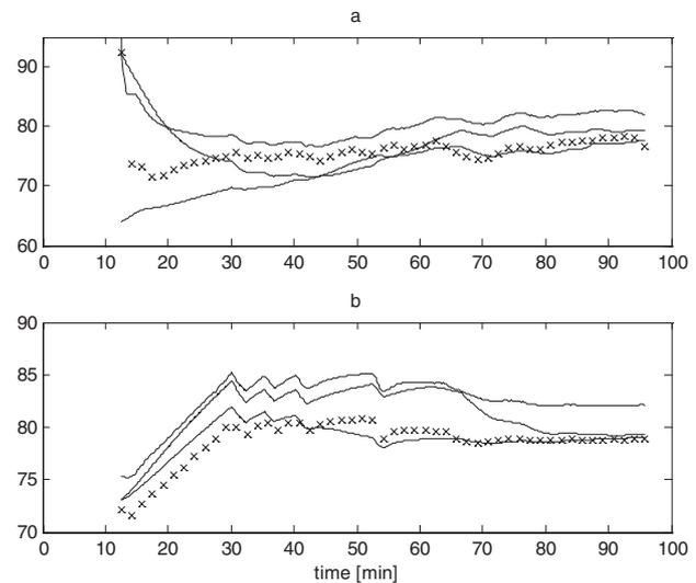
**Figure 6.** Validation stage. Process output predictions by the hybrid model (solid line), the analytical model (dotted line) and ANN model (dashed line) compared with industrial process data (x line).
