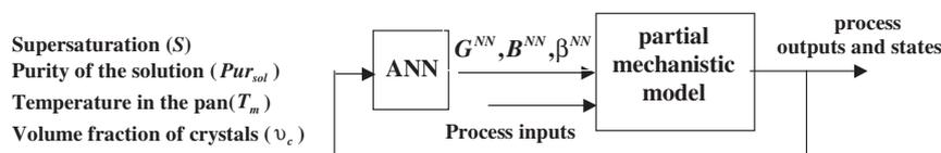
Figure 3. KBHM structure of sugar crystallization process.
