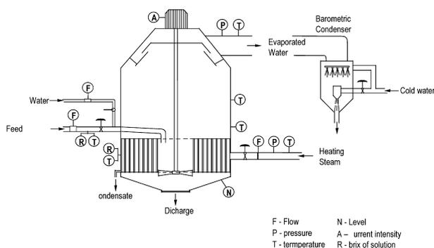
Figure 1. Industrial setup for a batch sugar crystallizer.
