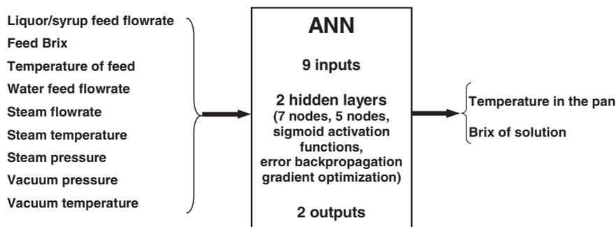
Figure 2. Data-driven model structure of sugar crystallization process.
