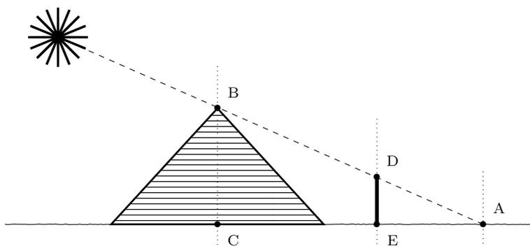
FIGURE 2 Thales' shadow measurement setup
