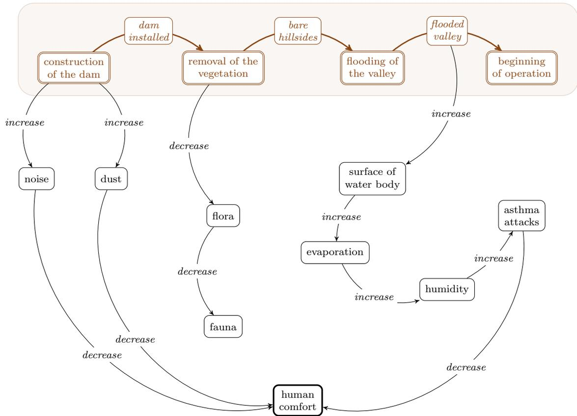
FIGURE 3 Hybrid diagram with the project CPD in the upper part (boxed, in colour), and the impact analysis DCD in the lower part (in black)
